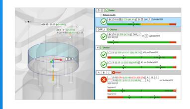
EVOLVE **Design** helps designers apply and verify GD&T (GPS) specifications by proofing the callouts and providing guidance directly from the standards.
