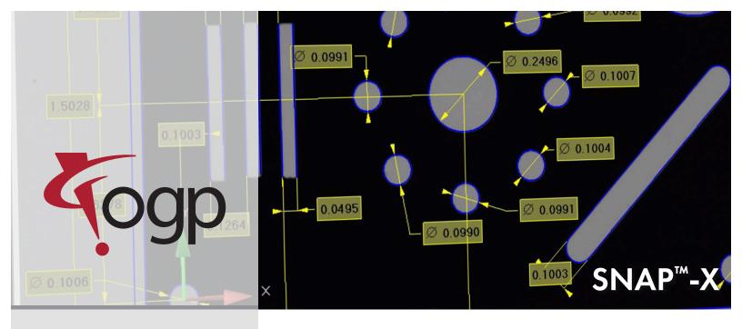
**SNAP-X** is a powerful metrology software program with a simple user interface. Three functions allow for a range of different uses – from fast walk-up measurement, to advanced GD&T analysis.
